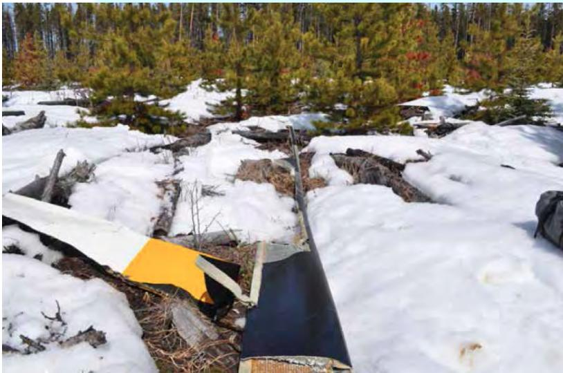
Image of the main rotor blade at the accident location
